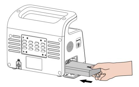
FIGURE 16 Install the battery
