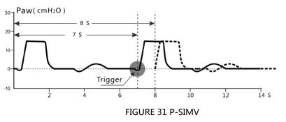
Note: the activation mode in T5 ventilator is pressure activation mode.
