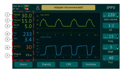
FIGURE 35 Ventilation Parameters
